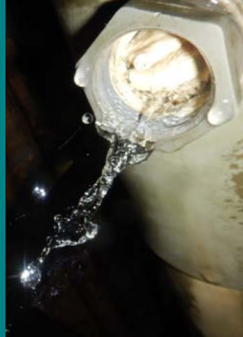
Water distribution nozzle spray clogged by sulfur and silica deposit
