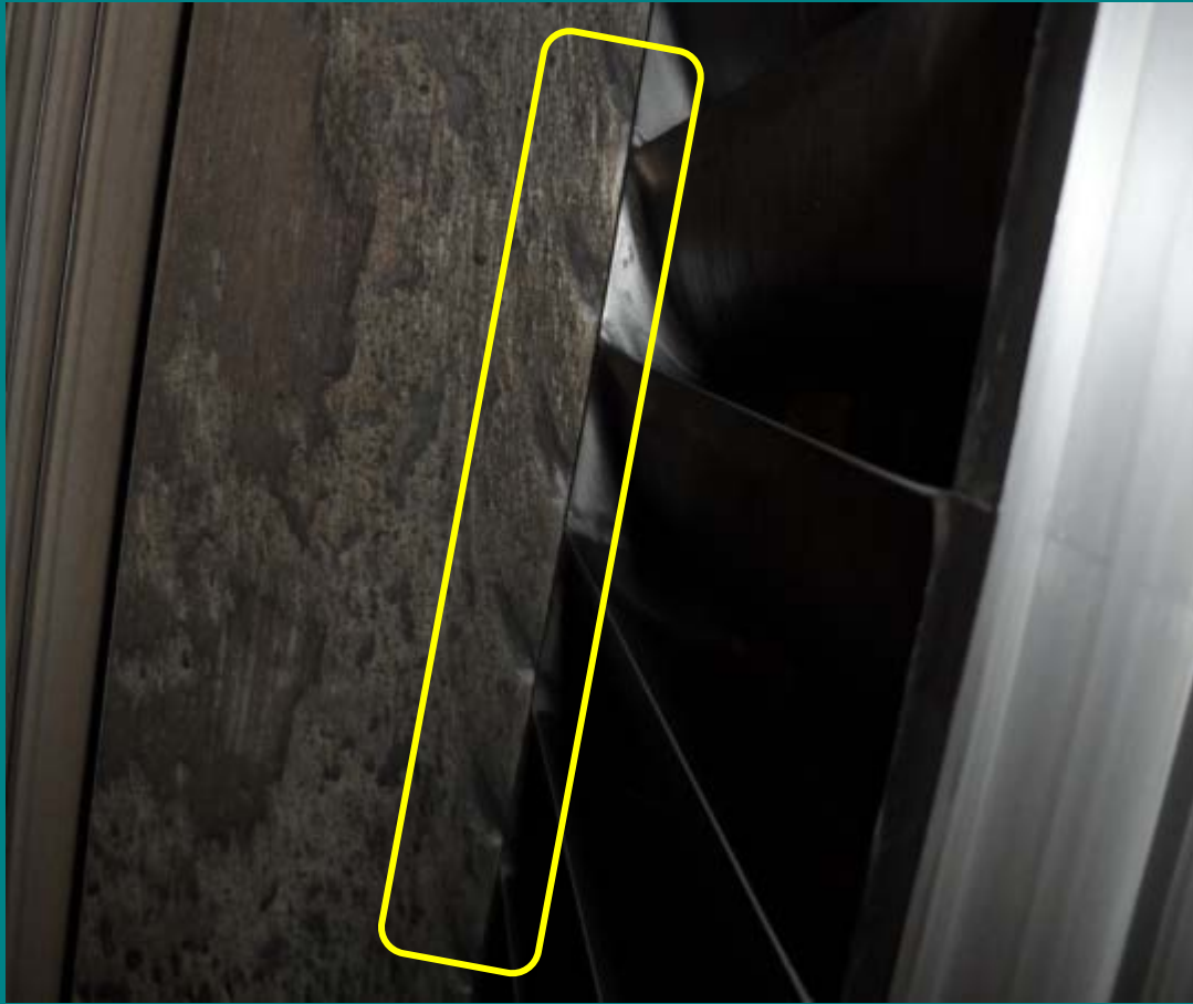
Erosion on turbine rotor
