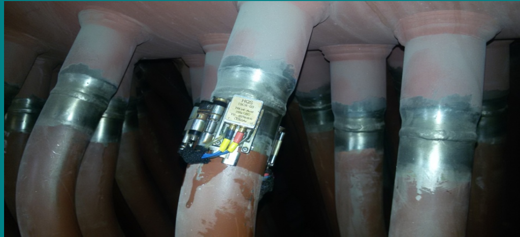
Ultrasonic boiler tube weld
