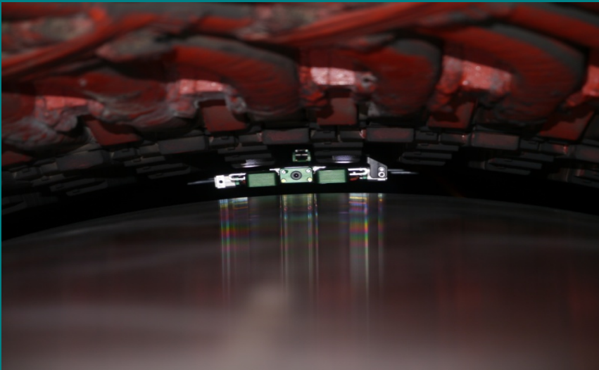
Generator testing robot with 4 miniature cameras
