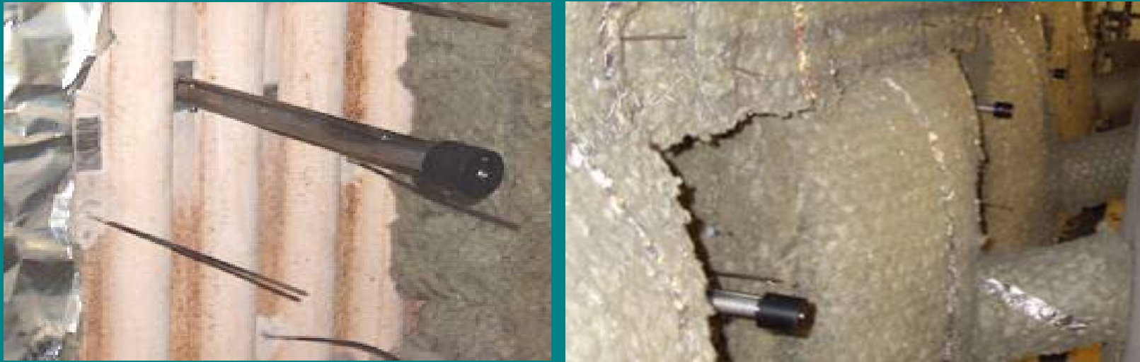
KEMWAT studs with fixed UT sensor
