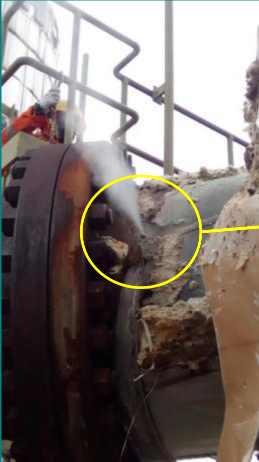
Pinhole leakage in weldment of pipeline
